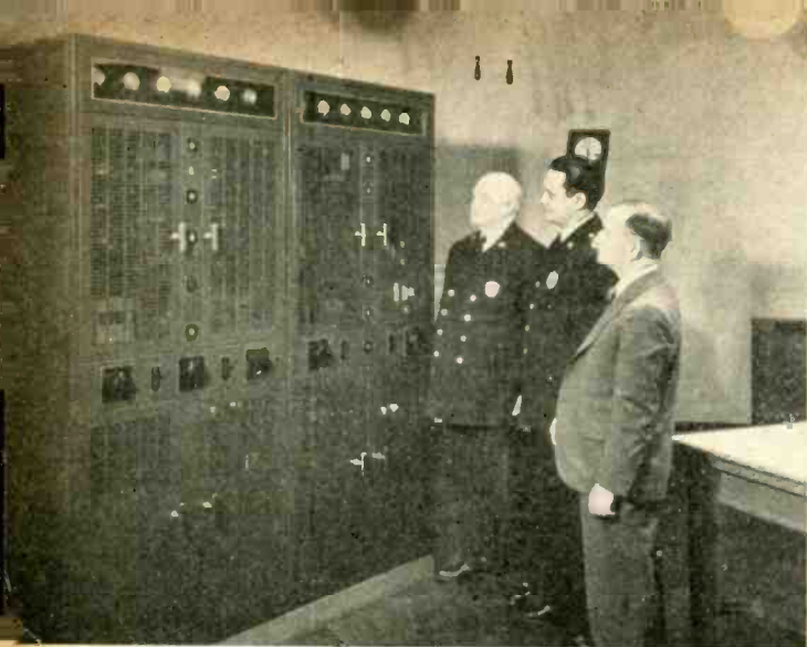
(Left). First New York City police radio transmitter was installed at Centre Street headquarters by Western Electric in 1932. Here Superintendent Allan and Assistant Superintendent Morris of the Telegraph Bureau view the 500-watt a-m transmitter with Chief Engineer Rochester. (Right). The 300-meter Centre Street transmitter, WPY, for communication with ships.
